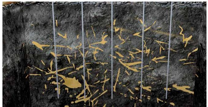
For this procedure, steel tubes (lances) with tips are rammed into the soil. Basically, there are two different variants:
